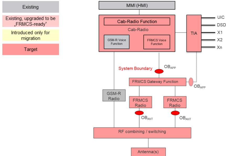
Figure 16: Cab Radio Variant 4b – New Cab Radio (Dual Mode, Option 3)
