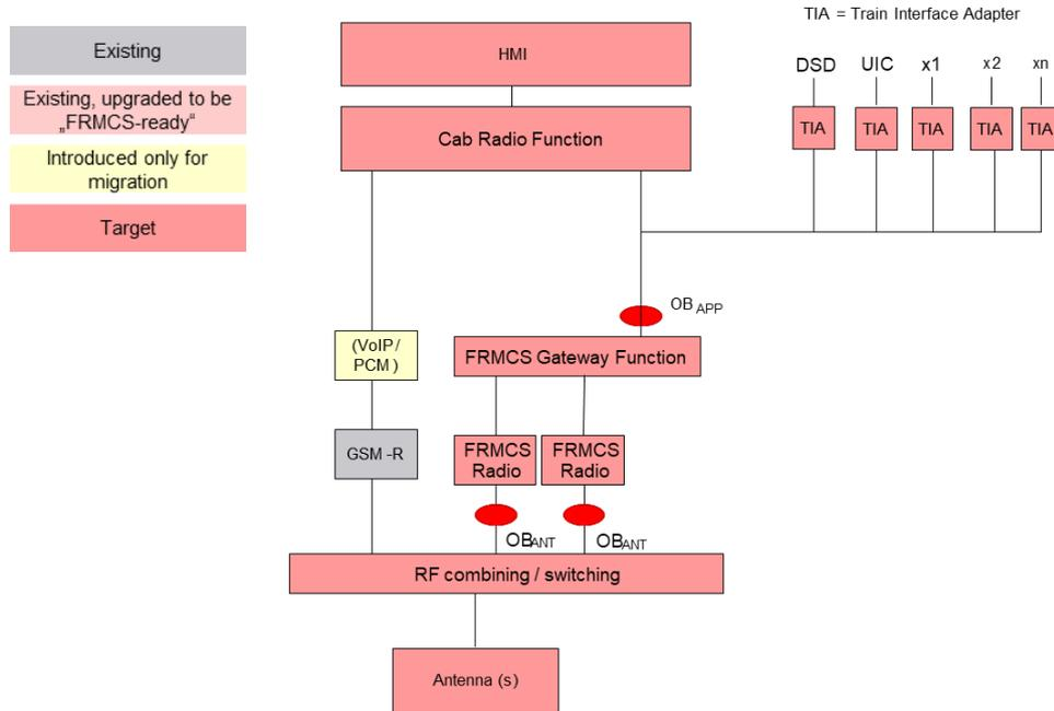
Figure 14: Cab Radio Variant 3 – New Cab Radio (Dual Mode, Option 2)
