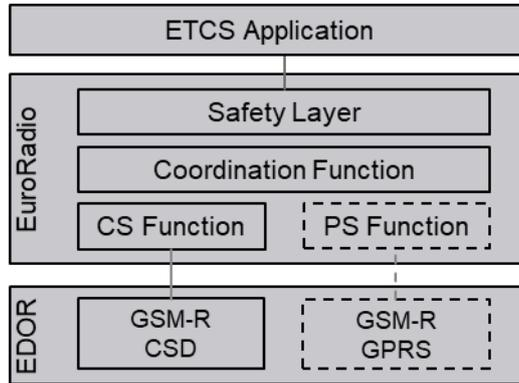
Figure 2: Functional block of existing ETCS OBU<sup>1</sup>
