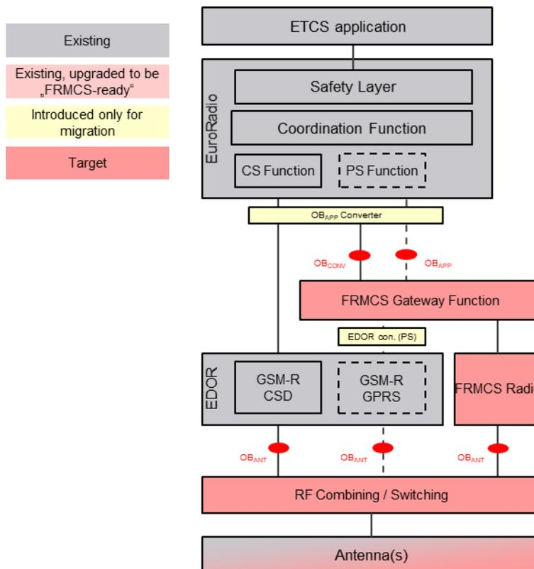
Figure 6: ETCS Variant 2 - Existing ETCS OBU with CS bypass and PS conversion.
