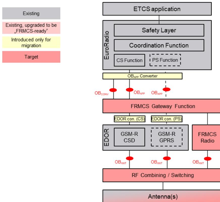
Figure 3: ETCS variant 1a - Existing ETCS OBU with CS and PS conversion.<sup>2</sup>
