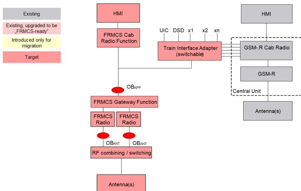
Figure 12: Cab Radio Variant 1 - Existing GSM-R Cab Radio + single Mode FRMCS Cab Radio
