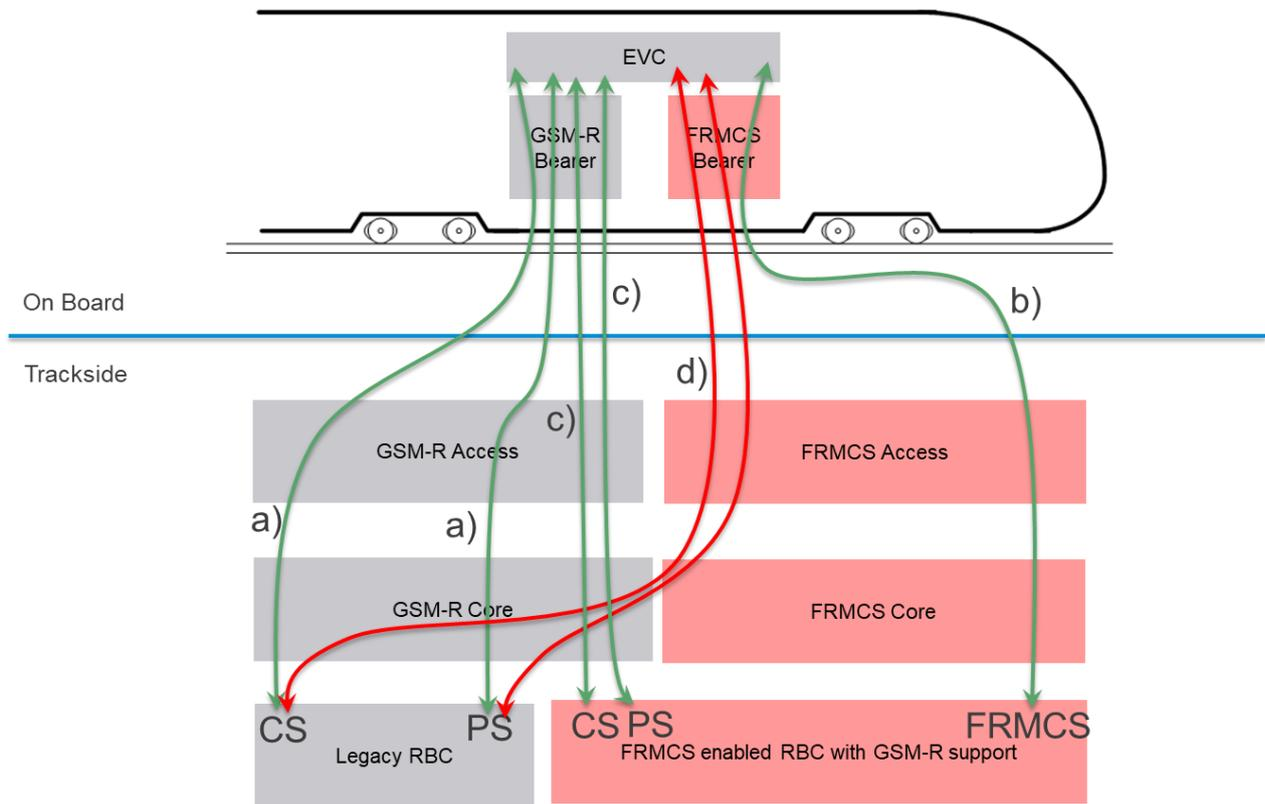
Figure 11: ETCS interworking on-board and trackside
