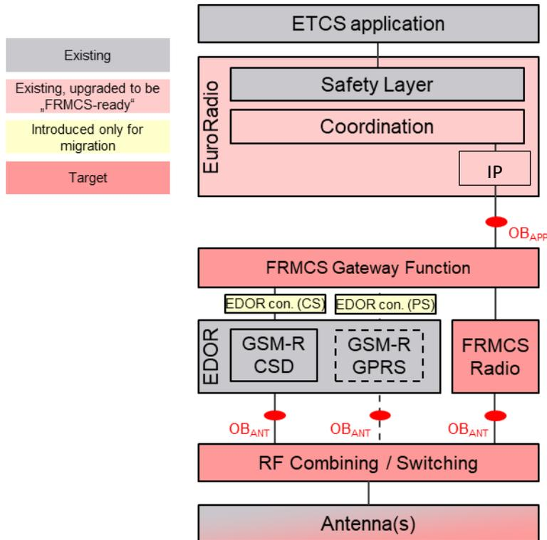
Figure 8: ETCS Variant 4 - Modified Euroradio reduced to FRMCS support.<sup>5</sup>
