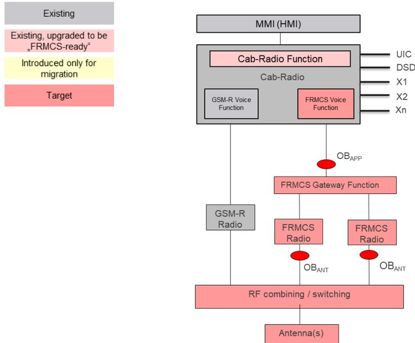
Figure 15: Cab Radio Variant 4a – New Cab Radio (Dual Mode, Option 3)
