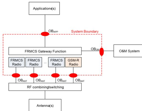
**Figure 1: Functional Architecture of FRMCS On-board System**
