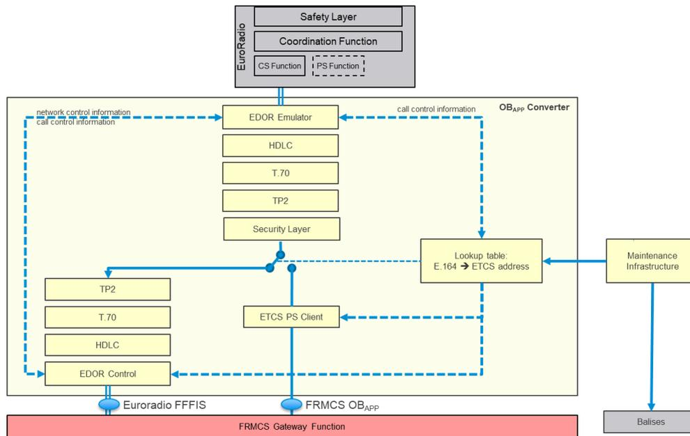
Figure 4: Detailed structure of the OB<sub>APP</sub> Converter for required for CS conversion
