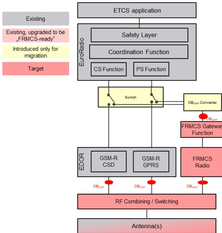
Figure 5: ETCS Variant 1b – Existing ETCS OBU with PS (or CS) Conversion/Bypass<sup>3</sup>
