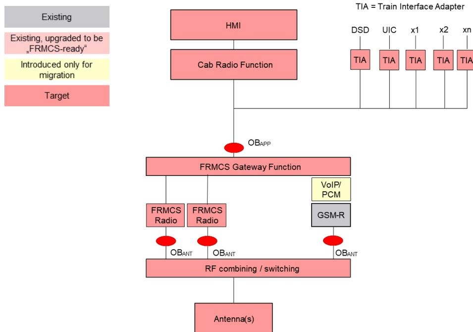
Figure 13: Cab Radio Variant 2 – New Cab Radio (Dual Mode, Option 1)
