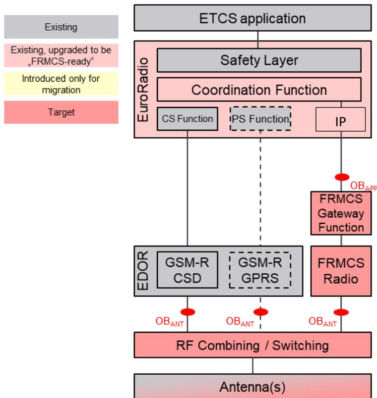
Figure 7: ETCS Variant 3 – Modified Euroradio with CS and PS bypass.<sup>4</sup>
