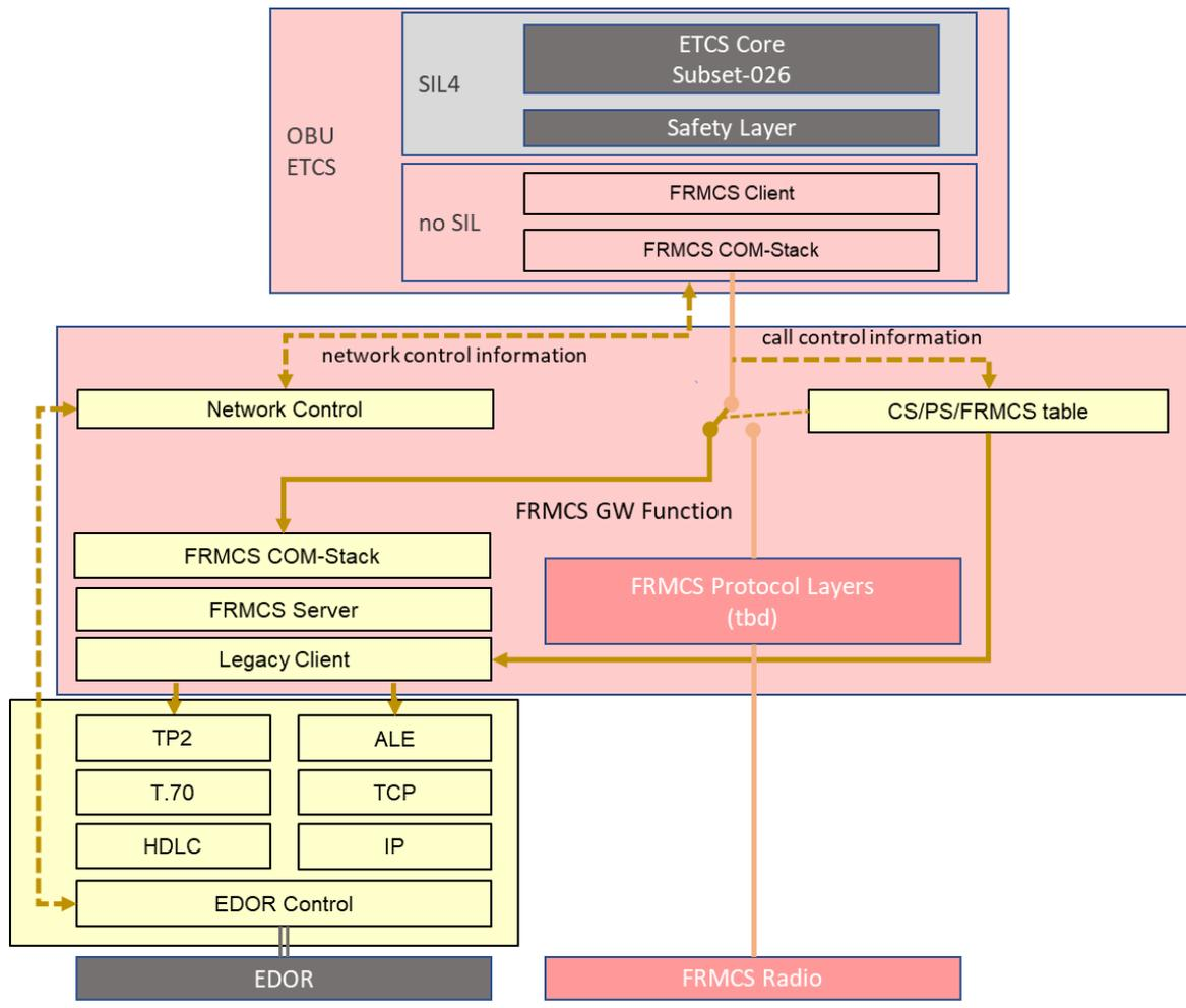
Figure 9: Detailed structure of the conversions needed for variant 4
