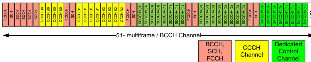
**Figure 2-14 Logical Channel sequence using combined channel setup - Downlink**
