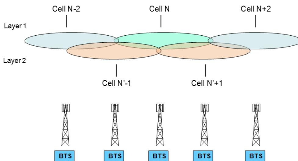
*Figure 2-12 Dual Radio Layer Coverage – with layer offset*
