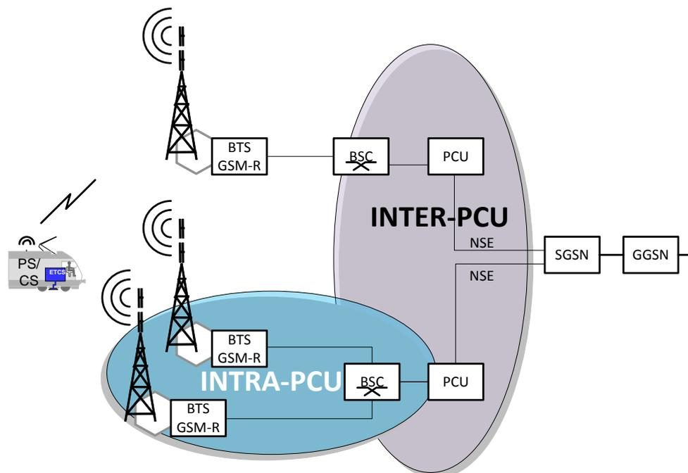
***Figure 4-2 PS-mode - Intra/Inter PCU architecture schematic***
