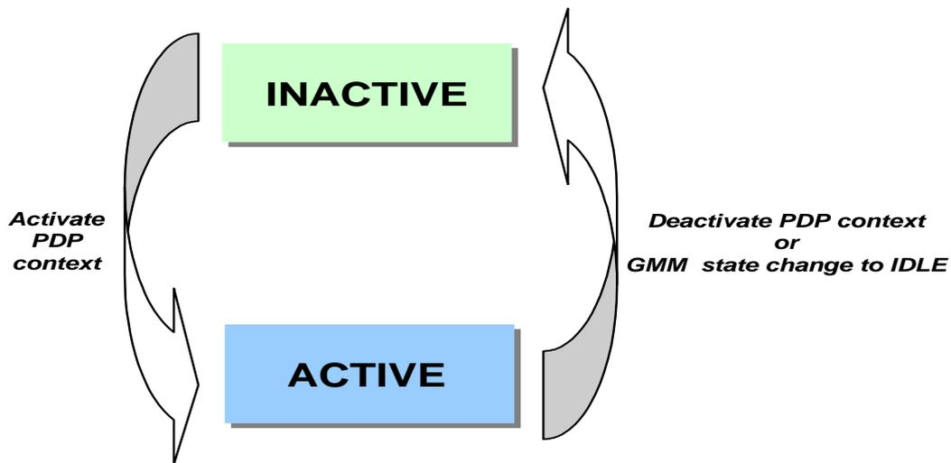
**Figure 8-1 PS-mode - Functional PDP state model**
