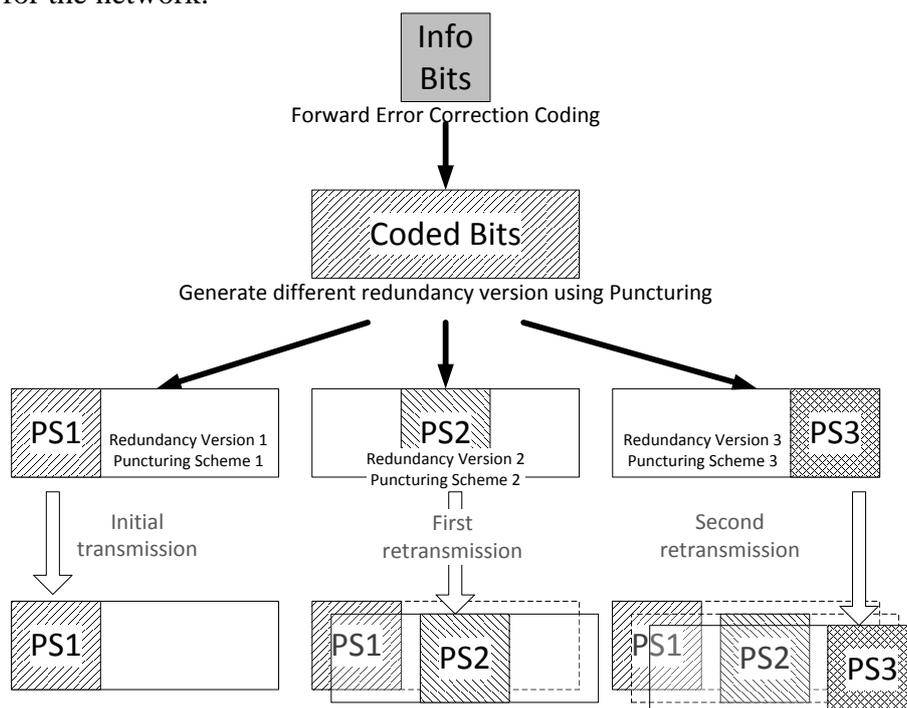
***Figure 2-8 Incremental redundancy principle***
