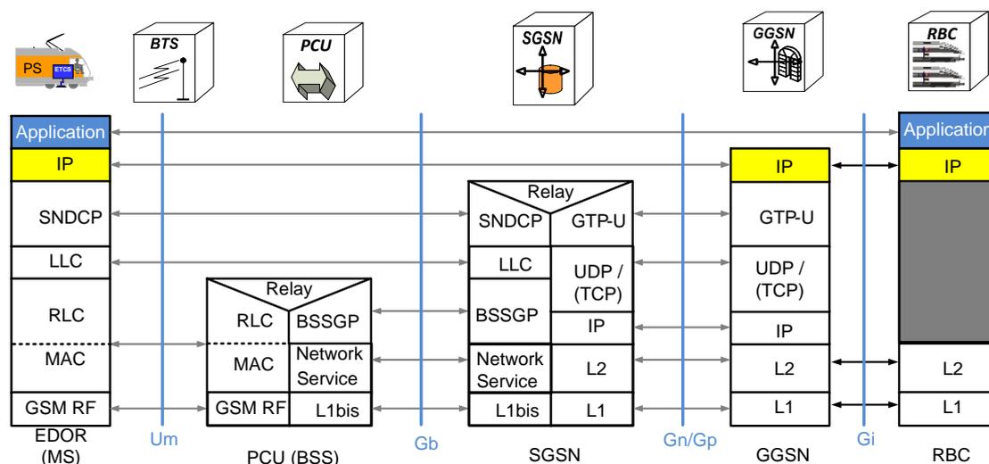
**Figure 2-2 Overview GPRS protocol stack – User Plane**
