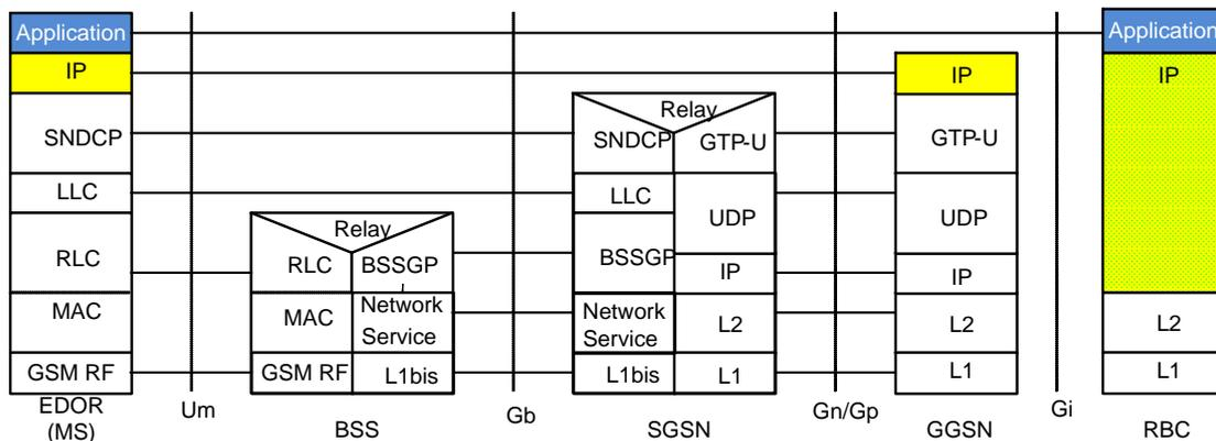
*Figure 2-5 GPRS User Plane protocol stack*
