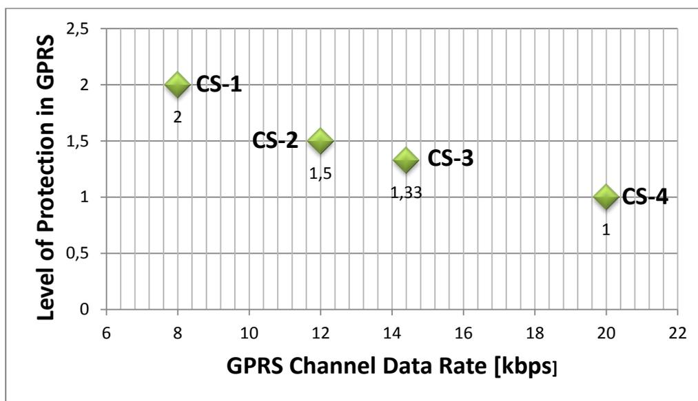
***Figure 2-6 Link between FEC and the resulting Channel Data rate in GPRS***
