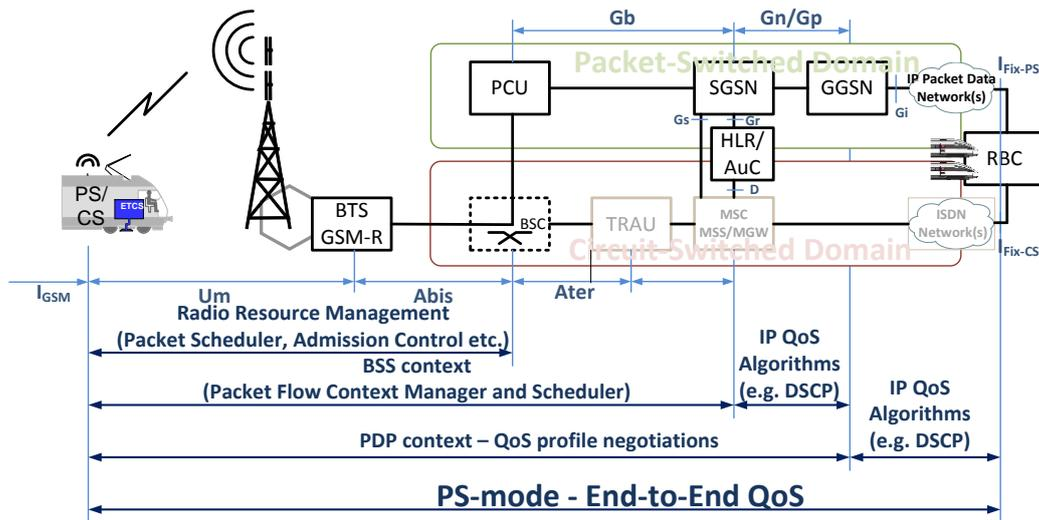
***Figure 5-1 PS-mode - End-to-End Quality of Service***
