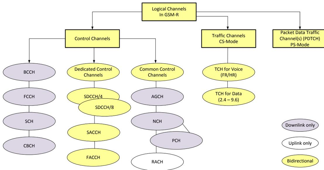
**Figure 2-13 Logical Channel Types applicable for GSM-R**
