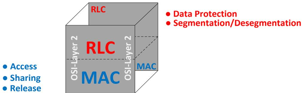
Figure 2-4 GPRS Protocol Stack - RLC/MAC transport functions
