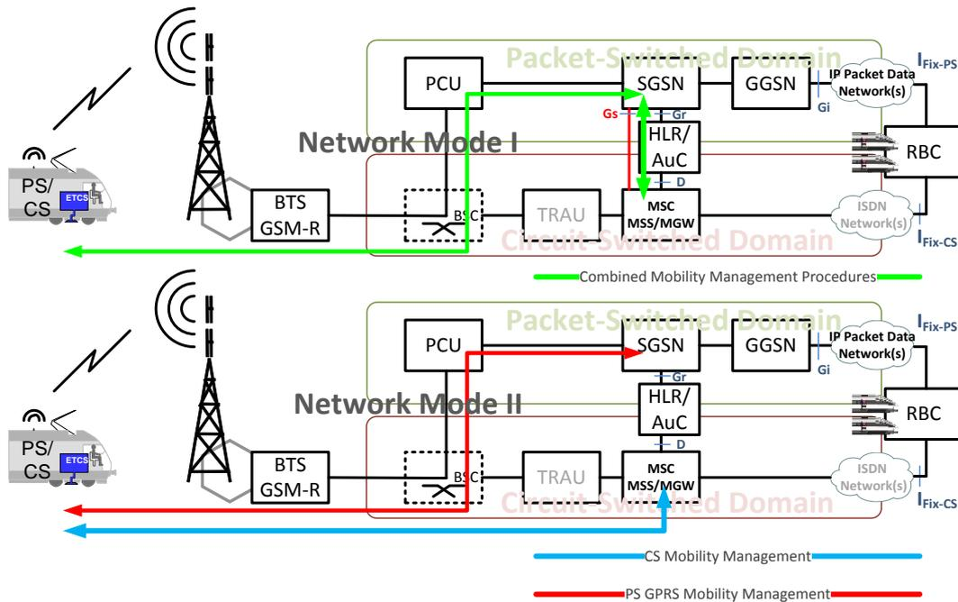
**Figure 8-2 GPRS Network Modes of Operation**
