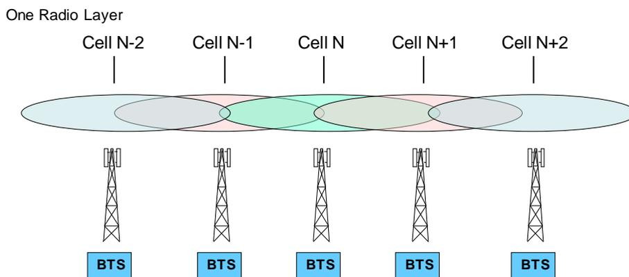
*Figure 2-10 Single radio layer architecture – extended adjacent cell overlapping*
