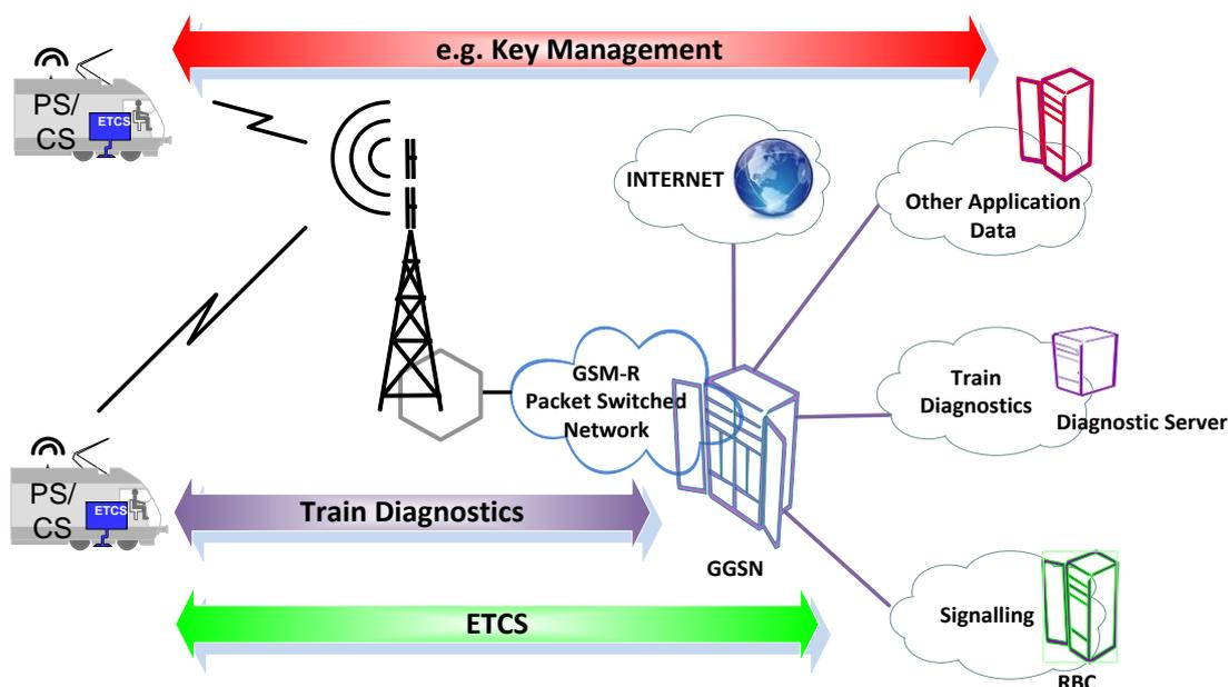
***Figure 8-4 Basic Security in PS-mode***
