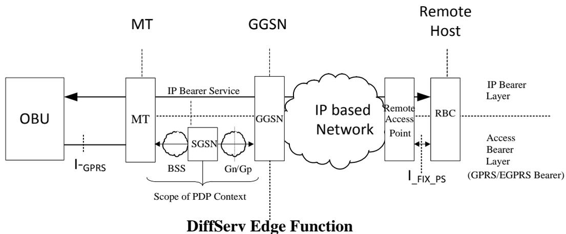
***Figure 5-3 PS-mode - QoS mapping between GPRS and IP based networks***
