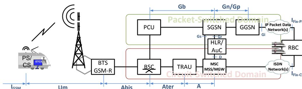
**Figure 2-1 GSM-R logical network architecture including CS- and PS-Domain**
