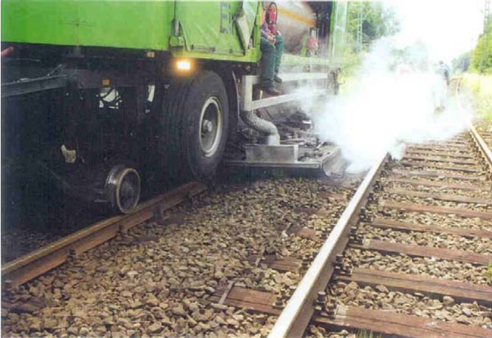
Picture 42 and 43: Wet steaming machine used in Germany: rail-road vehicle (left) and the one used in Switzerland and Austria: track-bound vehicle (right)
