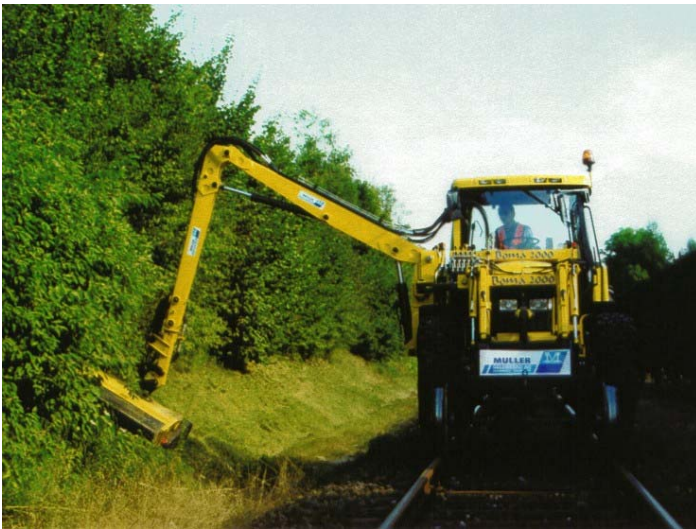
Picture 24: mowing with rail-road vehicle
