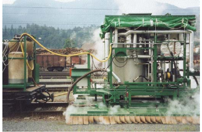
Picture 42 and 43: Wet steaming machine used in Germany: rail-road vehicle (left) and the one used in Switzerland and Austria: track-bound vehicle (right)
