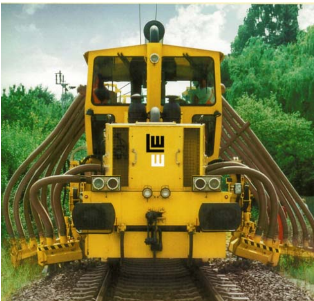
Picture 29 and 30: Mechanical weeding with WESPE (left) and with camulino (right)
