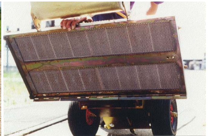
Picture 40 and 41: steel grids heated, only for use outside the track area
