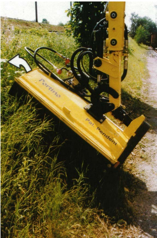
Picture 25: mulching: this machine blows the cut plants away from the transition area
